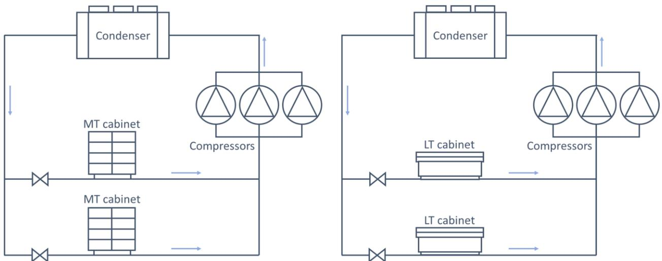
Figure 7. Simple direct expansion (DX) system.
