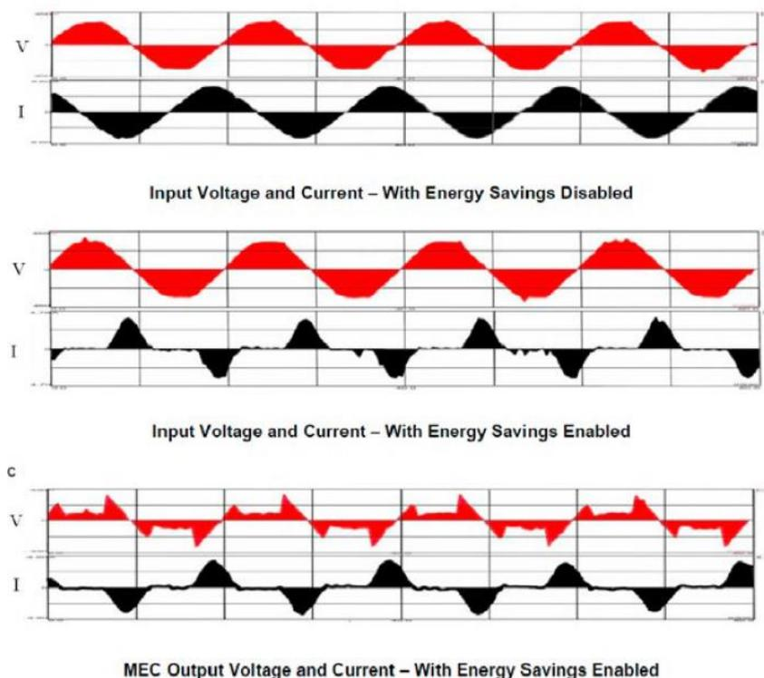
Figure 37. Current & voltage waveforms on single-phase motor both with and without energy savings (Envirostart).
