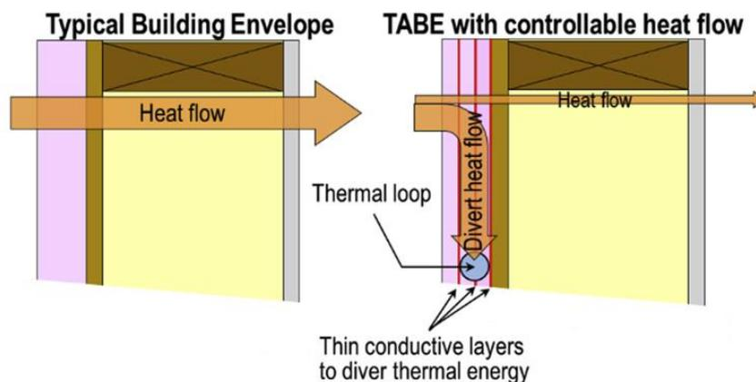
Figure 51. Thermally anisotropic building envelope.
