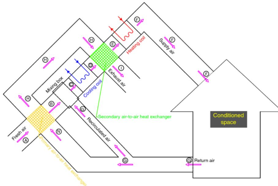
Figure 45: Simplified schema of an air handling unit (AHU) and a conditioned space (e.g. building) (Kalbasi et al., 2020)
