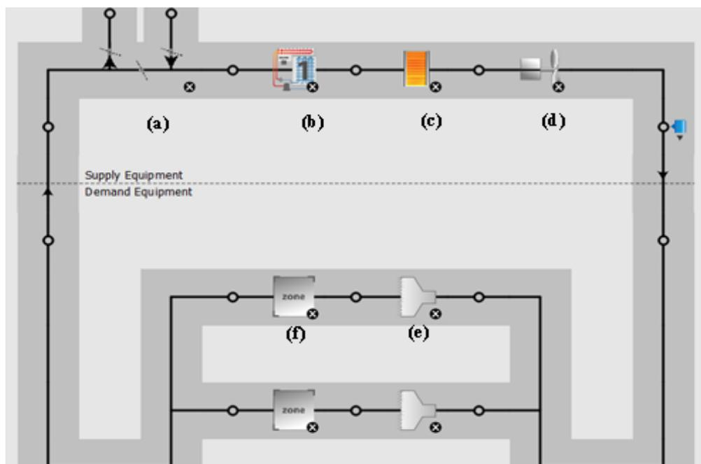
Figure 57. Adding a typical HVAC system for the MS supermarket: (a) Outside air system, (b) Cooling coil, (c) Electric heating coil, (d) Fan, (e) Zone terminal units, (f) Zone
