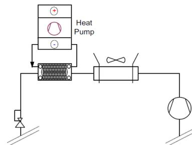
Figure 50: Simplified scheme of a heat recovery by means of a heat pump integrated after the aircooler (Sawalha, 2013)
