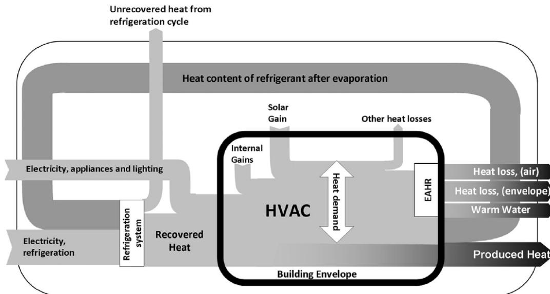
Figure 44: Energy flow diagram of a supermarket including heat recovery (Galvez-Martos et al., 2013)
