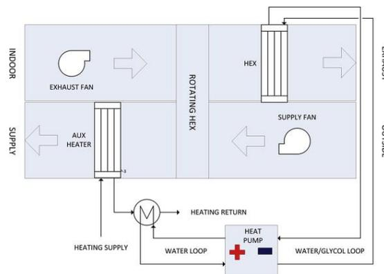
Figure 48: Simplified schema of an AHU with an energy wheel and an additional heat recovery with a heat pump (Wallin and Claesson, 2014)
