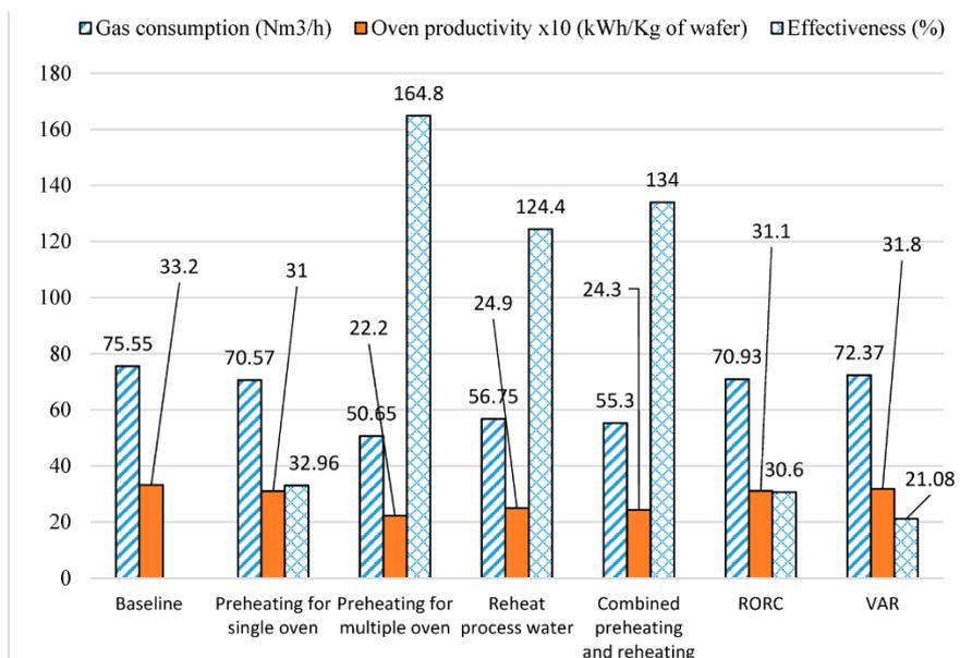
Figure 40. Comparison of heat recovery technologies based on oven's gas consumption, productivity and effectiveness. (taken from Mukherjee et al., 2020).
