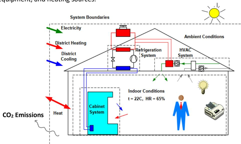
Figure 52. A conceptual scheme of the different subsystems in a supermarket and their interconnections, Taken from Arias (2005)
