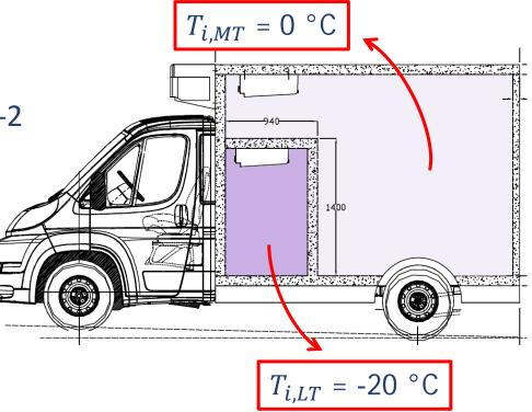
• Single-compression dual-temperature unit; back-pressure or ejector configuration for both MT and LT operation.
