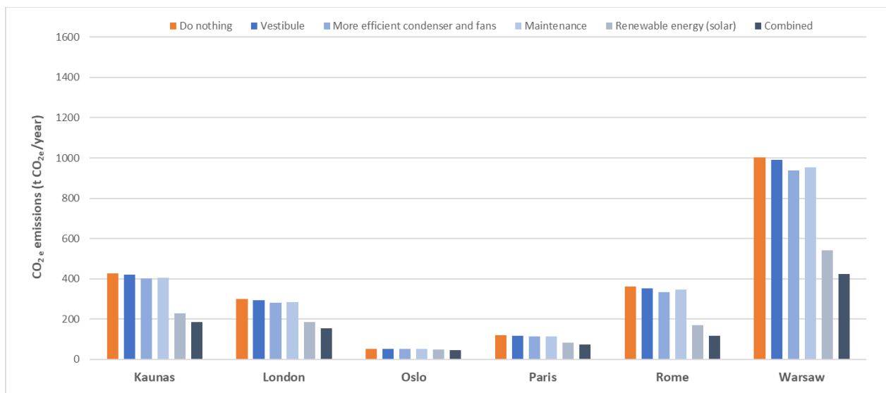
Figure 25. Impact on carbon emissions of retrofit options individually and applied together for the chilled store in the 6 locations.
