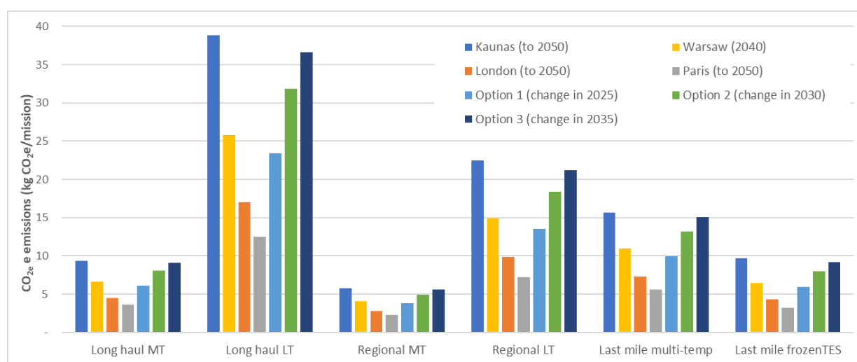
Figure 38. Accumulated carbon emitted between 2020 and 2050 for vehicle missions in Kaunas, London, Paris and Warsaw (for infiltration reduced, insulation improved, electrified R290 TRU).
