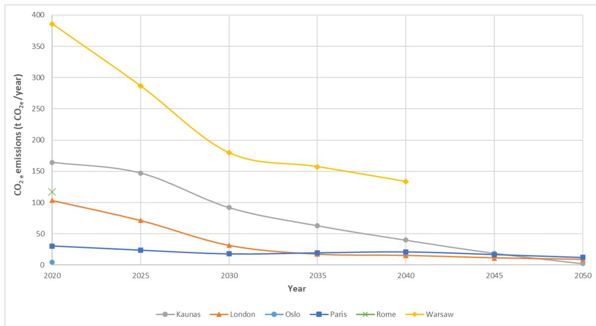
Figure 27. Impact on carbon emissions of the combined minor retrofit options for the 2,100 m<sup>2</sup> stores in the 6 countries from 2020 to 2040/50 (where data available).
