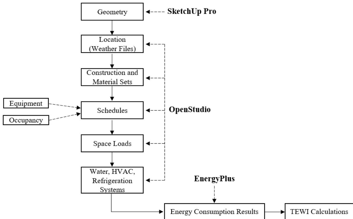
Figure 54. Methodology of work for modelling and simulating the case studies
