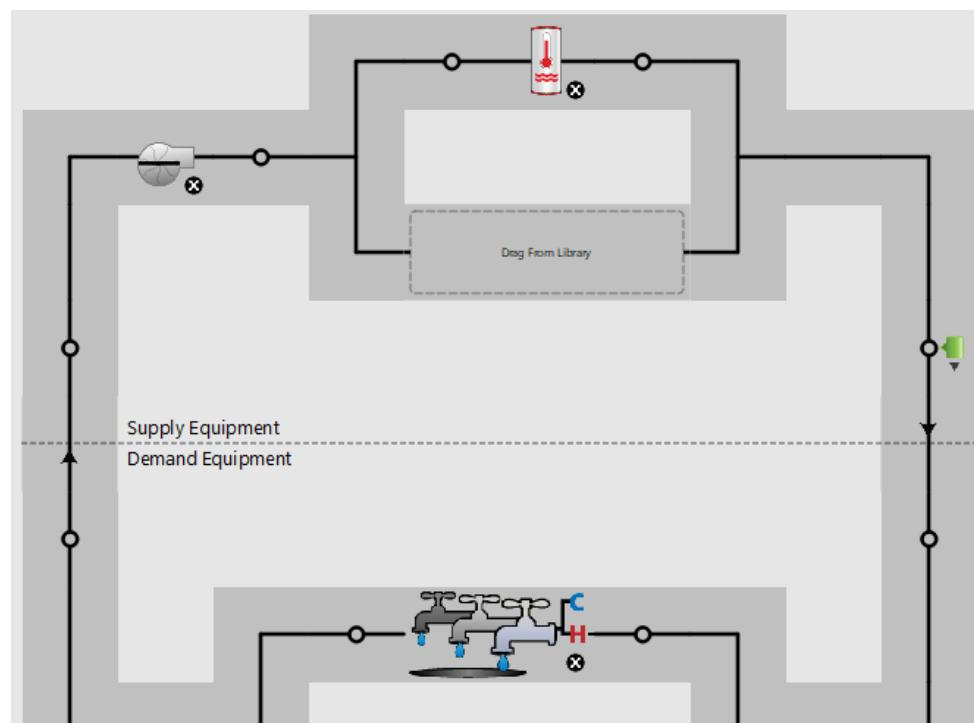
Figure 56. Adding a hot water loop for the MS supermarket
