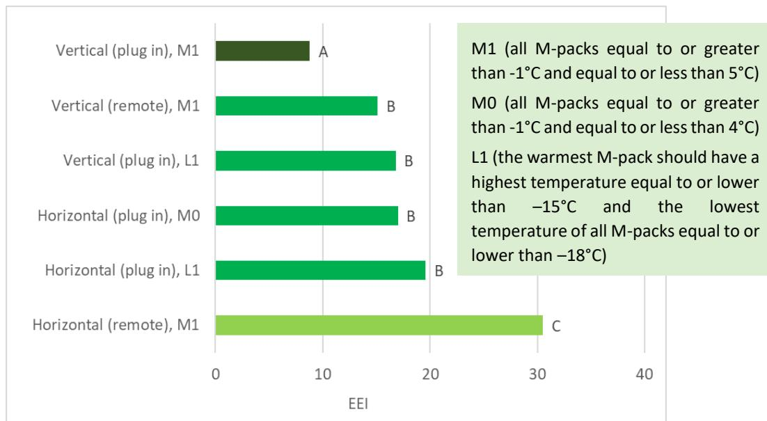
Figure 10. Most efficient refrigerated cabinets listed on Topten.
