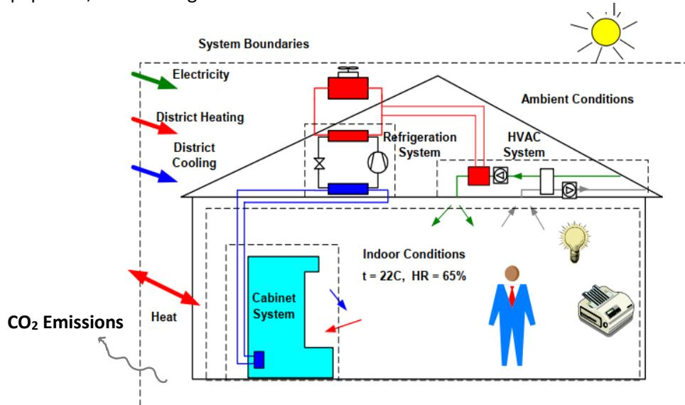
Figure 52. A conceptual scheme of the different subsystems in a supermarket and their interconnections, Taken from Arias (2005)
