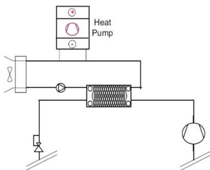
Figure 49: Simplified scheme of a heat recovery with a cascade system (Sawalha, 2013)
