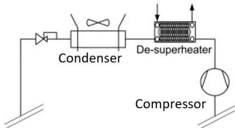
Figure 47: Simple scheme of a direct heat recovery solution via a desuperheater (Sawalha, 2013)
