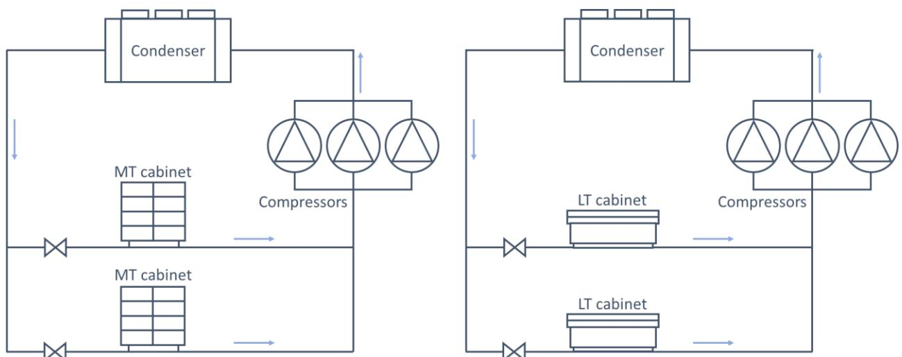
Figure 7. Simple direct expansion (DX) system.
