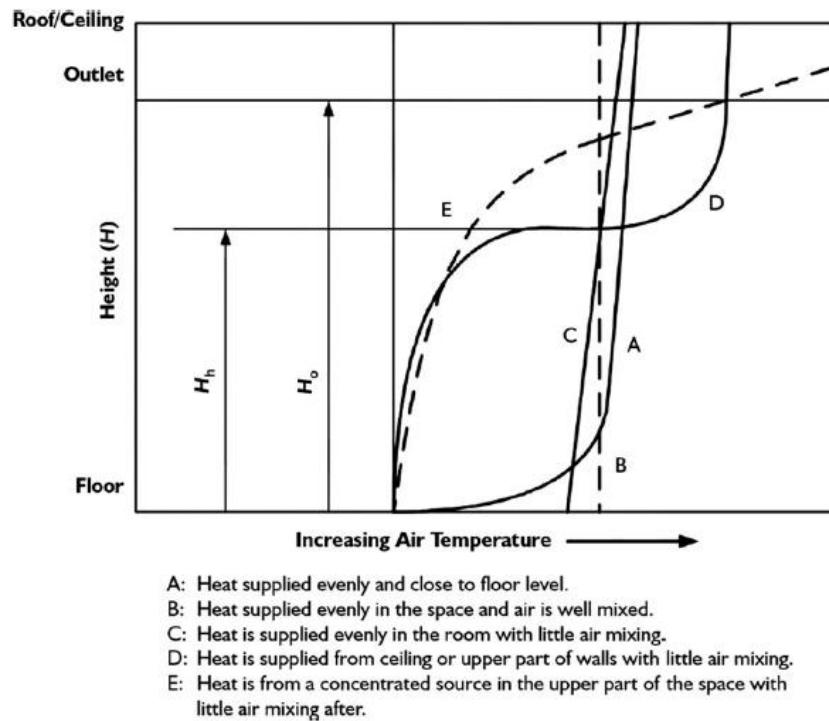
*Figure 43. Qualitative characteristic curves of thermal stratification, retrieved from Wang et al. (2019)*
