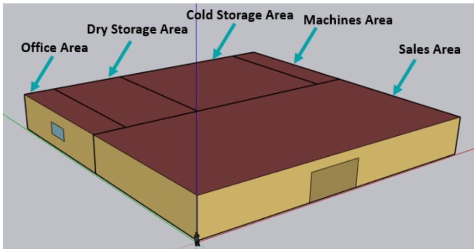
Figure 55. Geometry of the MS supermarket with its space types
