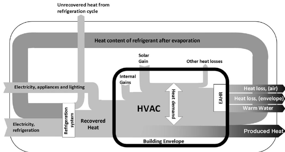
Figure 44: Energy flow diagram of a supermarket including heat recovery (Galvez-Martos et al., 2013)
