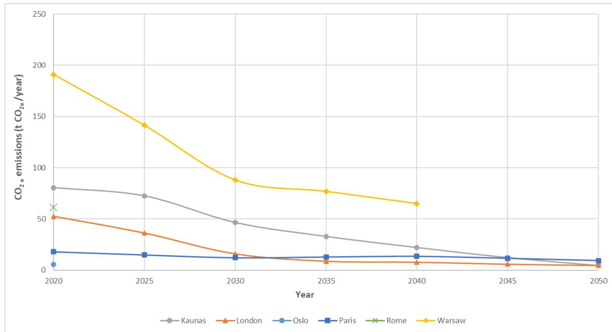
Figure 28. Impact on carbon emissions of the combined minor retrofit options for the 600 m<sup>2</sup> stores in the 6 countries from 2020 to 2040/50 (where data available).
