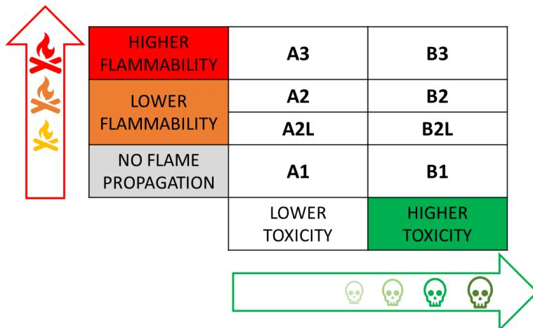
Figure 3. Toxicity and flammability classification of refrigerants.
