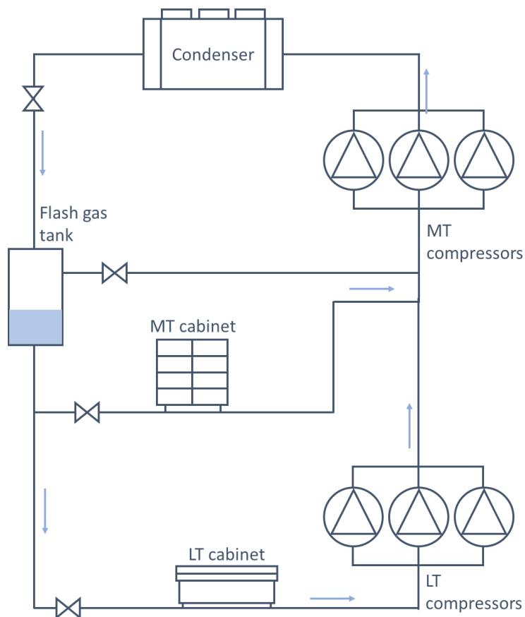
Figure 58. Adding a refrigeration system for the MS supermarket
