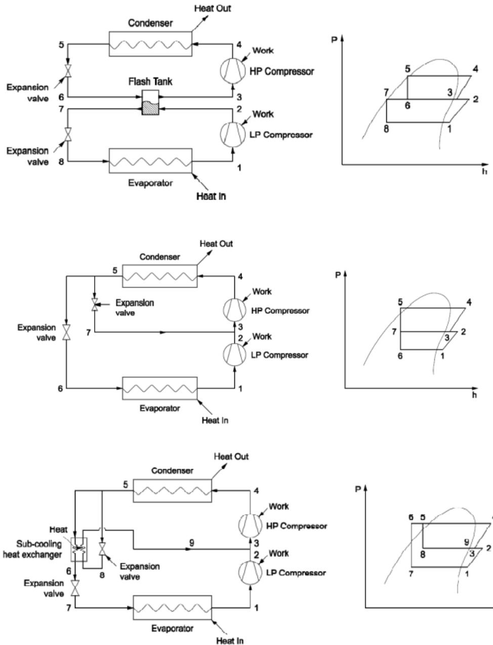
Figure 39. Three two-stage system configurations [Torrella et al (2009)].
