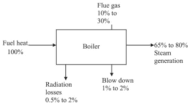
Figure 42. Typical heat balance of a boiler (Barma et al., 2017)
