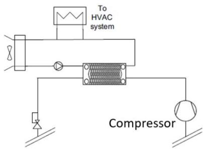
Figure 46: Simple scheme of a direct heat recovery solution via an intermediate circuit and a floating condensation pressure (Sawalha, 2013)
