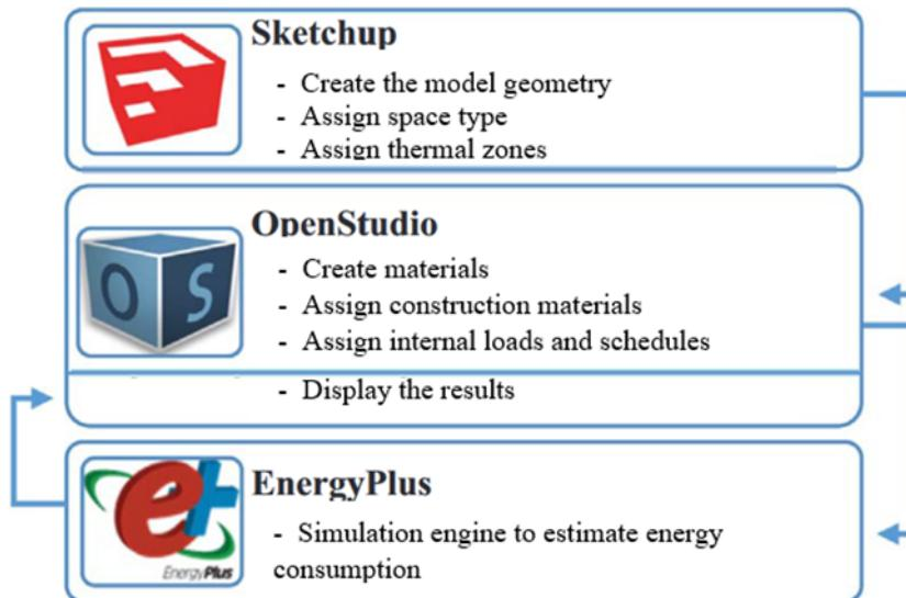
Figure 53. Workflow for modelling and simulating a building
