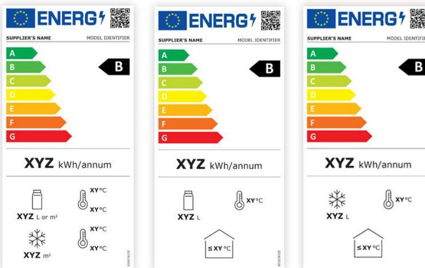
Figure 6. Energy label for (left to right: refrigerating appliances with a direct sales function, except for beverage coolers and ice-cream freezers, beverage coolers, ice-cream freezers.
