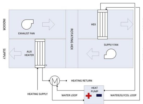
Figure 48: Simplified schema of an AHU with an energy wheel and an additional heat recovery with a heat pump (Wallin and Claesson, 2014)
