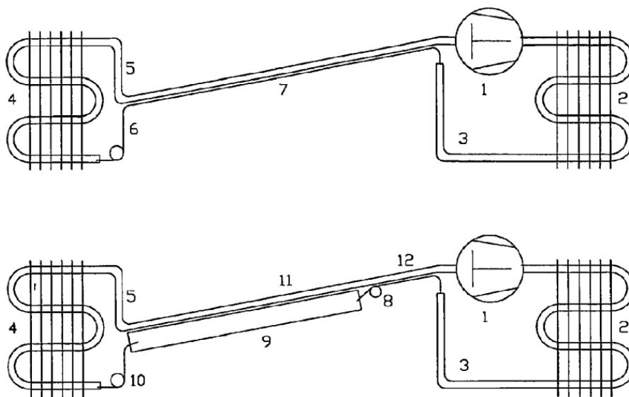
*Figure 38. TFC concept (upper diagram conventional capillary system, lower diagram TFC system)*
