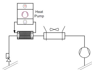
Figure 50: Simplified scheme of a heat recovery by means of a heat pump integrated after the aircooler (Sawalha, 2013)
