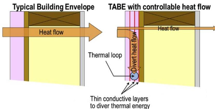
Figure 51. Thermally anisotropic building envelope.
