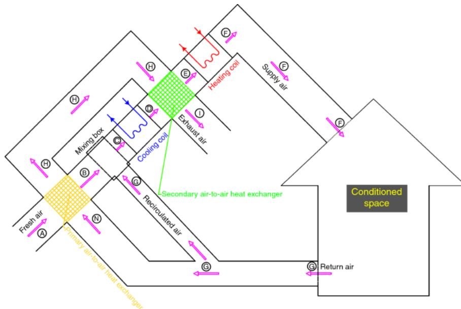
Figure 45: Simplified schema of an air handling unit (AHU) and a conditioned space (e.g. building)
