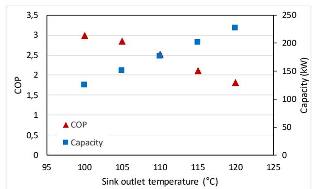
COPs and heat capacities at different heat sink outlet temperature
